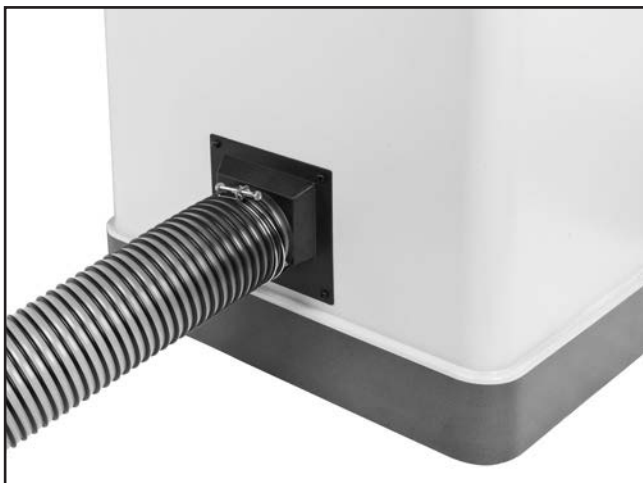
Figure 39. Example of dust hose attached to dust port.
